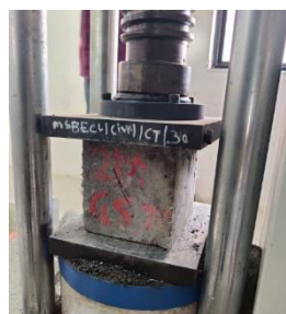
Fig. 2: Compressive Test of Cube Specimen
